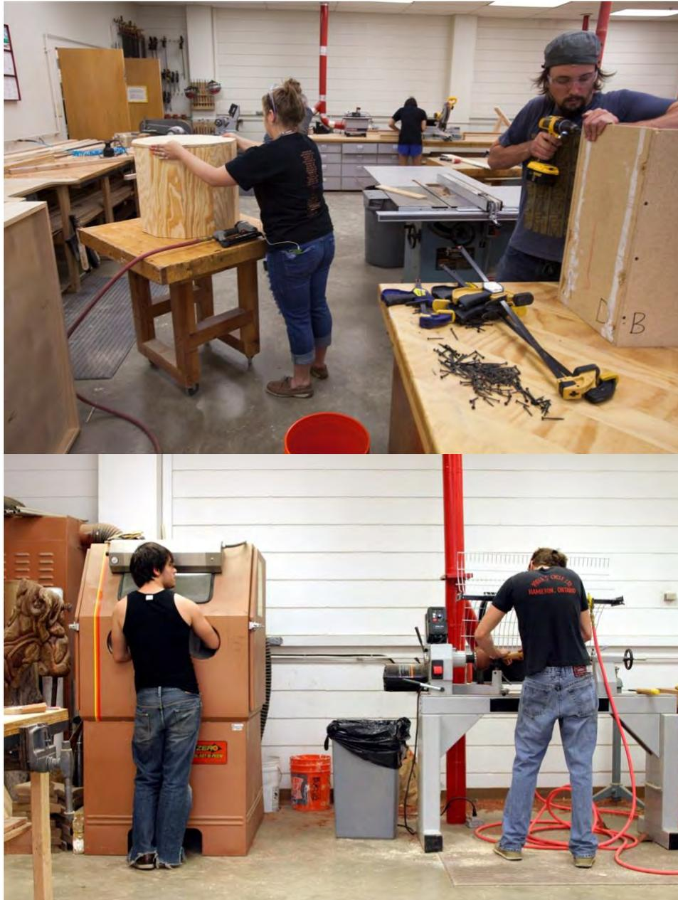
Across from the Serigraphy Print Lab, you'll find the Woodshop. The Woodshop is a well-equipped space with machines, manual and power hand tools, and miscellaneous equipment for working with wood and other materials. The shop's inventory includes a jointer and planer, table saws, bandsaws, routers, a mortising machine, a wood lathe, drill presses, a variety of hand tools, and more. During their freshmen year, students learn how to use these tools to complete projects!
